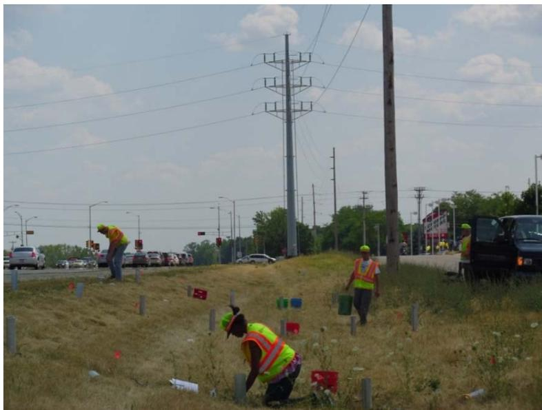
**Figure 1. Taking infiltration measurements using the MPD Infiltrometer in the swale located near Hwy 51, Madison, WI.**
