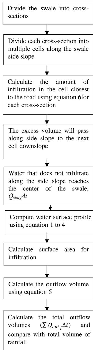
**Figure 4. Flow chart of the steps involved in runoff-routing model.**
